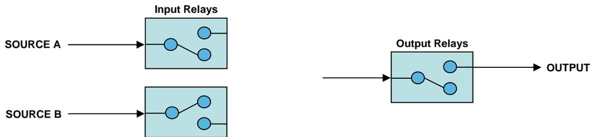
Firmware detects that source A is out of the user specified tolerance range. The input power from Source A is removed, then the output is disconnected. Crucial timing is controlled through the firmware.
